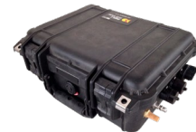
Depending on the on-site situation, place the measuring case and compressor and connect the MID cable and the compressed air supply.
